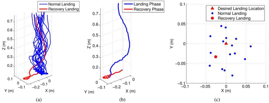
Figure 6: Partial trajectories of the aerial robot during seventeen landing trials (Fig. 6(a)). During one trial, the vehicle attempts and fails to land, causing it to enter a recovery phase before successfully landing (Fig. 6(b)). A scatter plot of the final landing locations is shown in Fig. 6(c).
