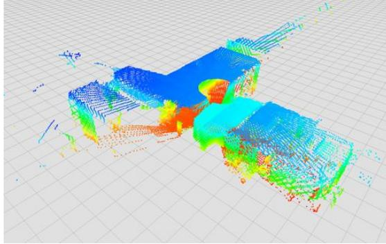
Figure 8: The 3D rotating laser scanner on the Kenaf generates feature-rich 3D point clouds. Here we show the full output from a single revolution of the scanner.
