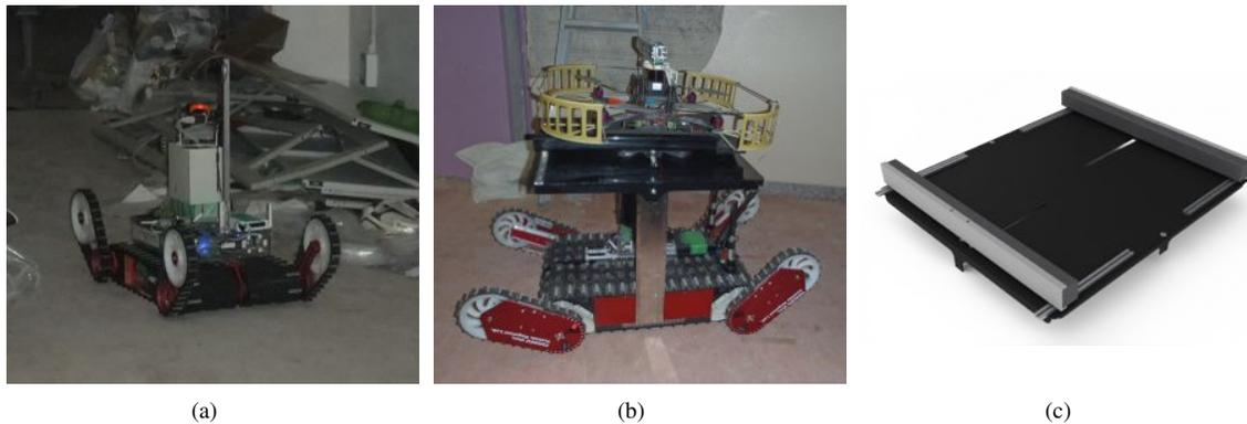
Figure 4: The three robots used in the experiments include the Kenaf (Fig. 4(a)) and Quince (Fig. 4(b)) tracked ground robots. Here we see the Quince transporting the Pelican between discrete sites of interest via the landing pad (Fig. 4(c)).
