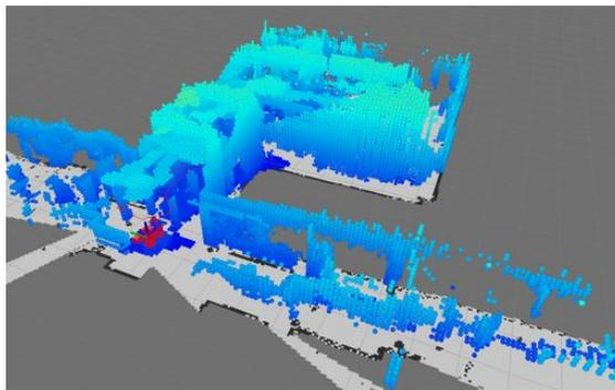
Figure 9: A representative 3D map generated by the aerial vehicle during flight. A 2D occupancy grid map is also generated at all times. The vehicle and its planned path are shown as a red mesh and line, respectively.
