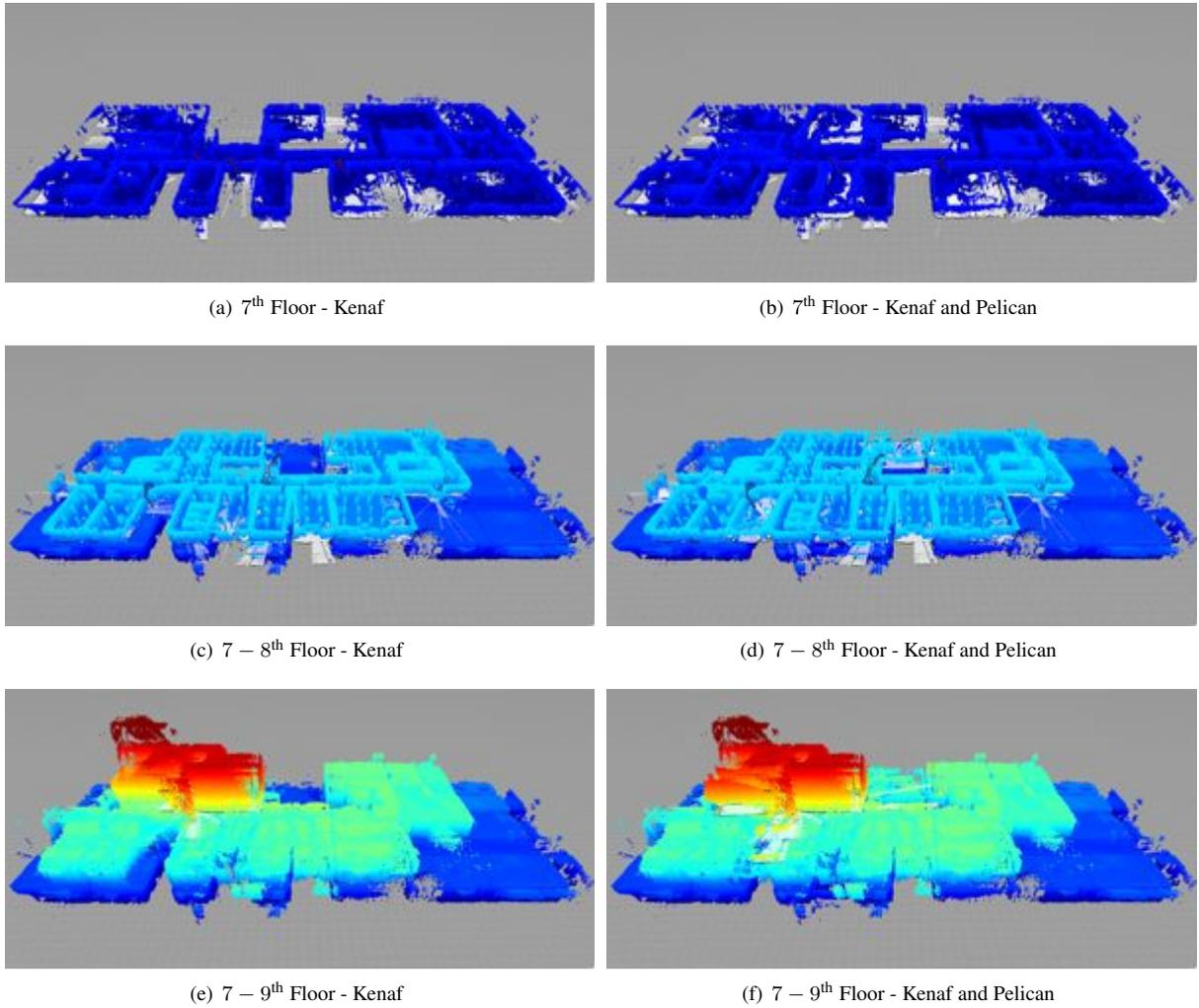
Figure 11: The 3D voxel grid maps generated during the experiment. The map resulting from the Kenaf sensor data is shown on the left while the merged maps resulting from both the Kenaf and Pelican sensor data are shown on the right.
