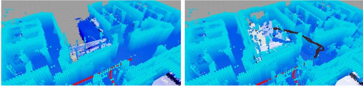
Figure 12: Merging the Kenaf and Pelican maps. The map generated by the Kenaf is shown on the left while the extended map via the Pelican observations along with the Quince and Pelican trajectories (red and black, respectively) are shown on the right.
