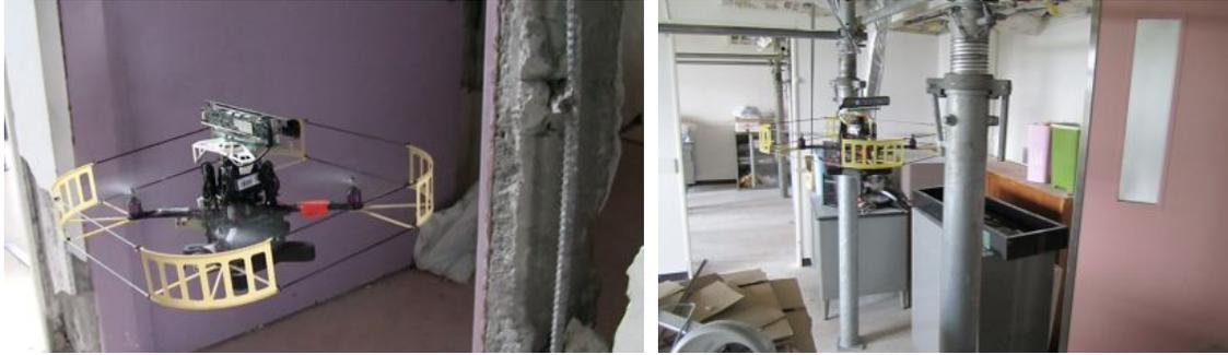
Figure 5: The aerial robot flies through cluttered regions of the environment that are inaccessible to the ground robot and builds a 3D map that will be merged with the maps made by the ground robot.
