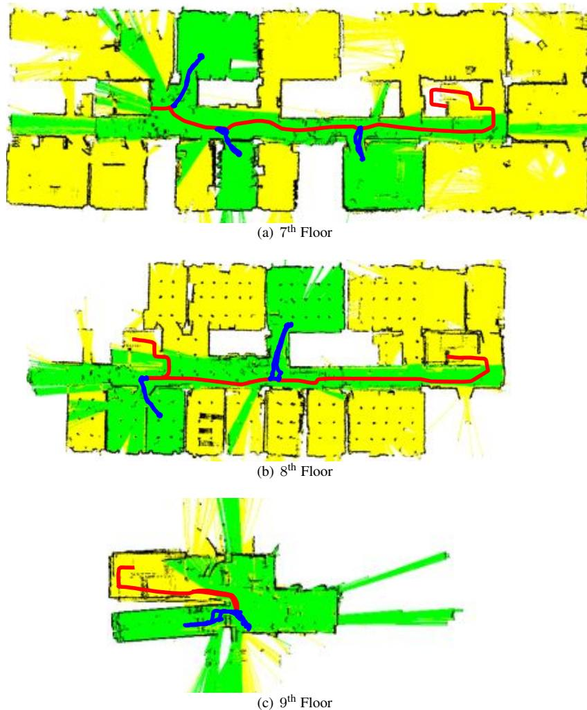
Figure 10: The 2D occupancy grid maps generated during the experiment of the 7<sup>th</sup>, 8<sup>th</sup>, and 9<sup>th</sup> stories of the Tohoku University Electrical Engineering Building. The contributions to the map made by the Kenaf are shown in yellow with an overlay of the contributions made by the Pelican in green. The path of the Quince is shown in red while the trajectory followed by the Pelican is depicted in blue.
