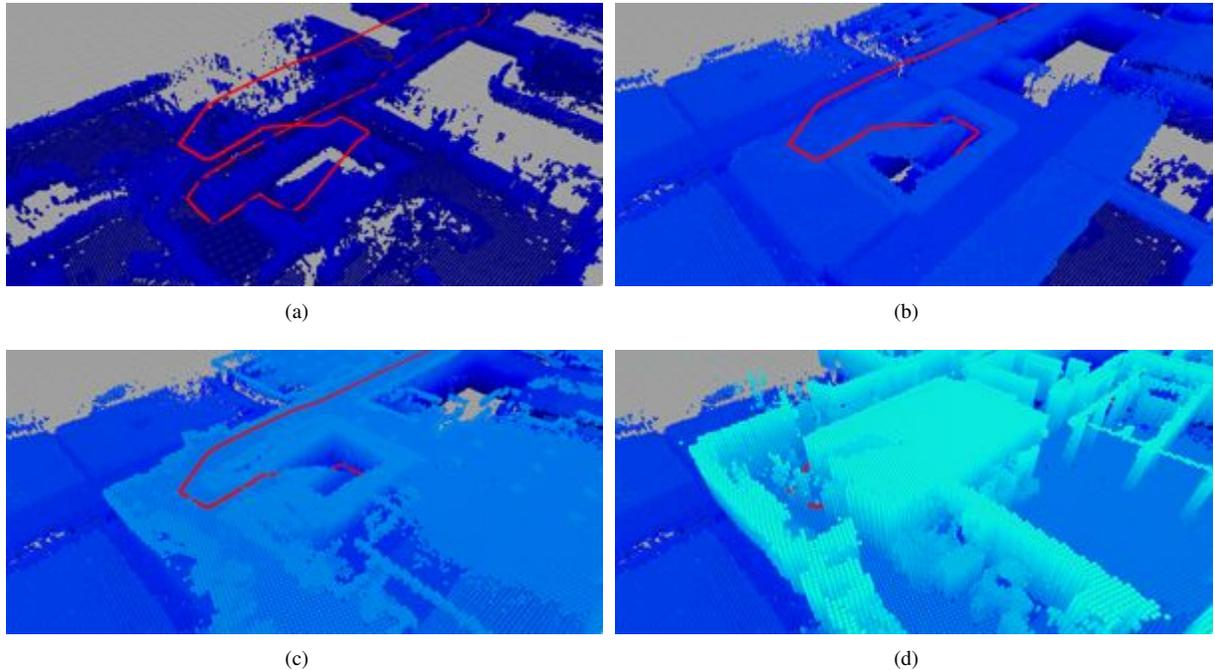
Figure 13: The 3D map generated for the stairwell traversed by the vehicles between the 7<sup>th</sup> and 8<sup>th</sup> floors showing various  $z$ -height levels of detail along with the trajectory followed by the Quince robot.
